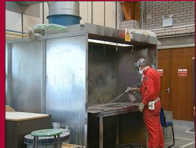
(Enclosure Contain and separate)
